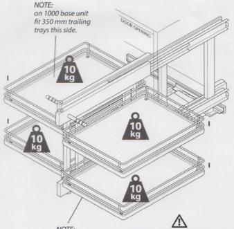
NOTE: on 1000 base unit fit 300 mm leading trays this side.
