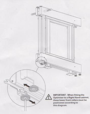
5 Lower slider unit onto runner carriage and attach the 6 nuts.
